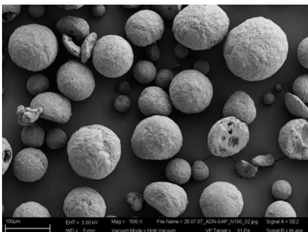
Figure 4: ADN-Prills coated with di-functional GAP
