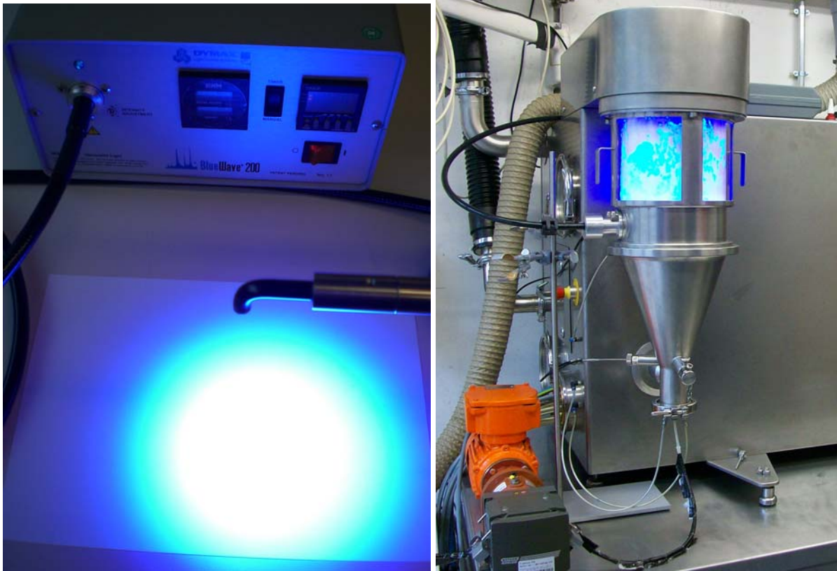
Figure 2: UV-point light source with orthogonal light guide (left). Fluidized bed vessel with implemented light source (right).
