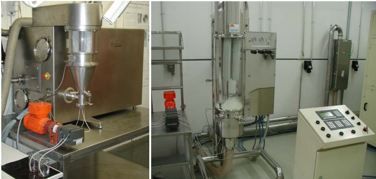
Figure 1: Laboratory-scale fluidized bed coating apparatus (Hüttlin, Mycrolab, left) and field-scale fluidized bed coating apparatus (Hüttlin, HKC5, right)
